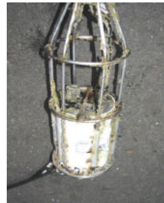
Figure 1: photograph of METOCEAN drifter 52197 in December 2005, roughly one week after its recovery during the CONGAS2 cruise. The subsurface sensor area is shown with noticeable algal fouling near the sensors.
