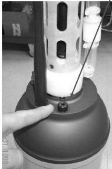
rotate counter –clockwise to unscrew plug.
