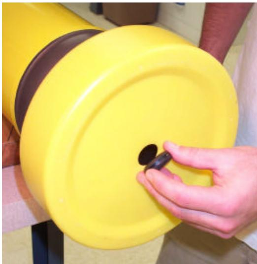
2. The minimum internal temperature of the float is -2.0 °C. If necessary, let float warm indoors before proceeding.
