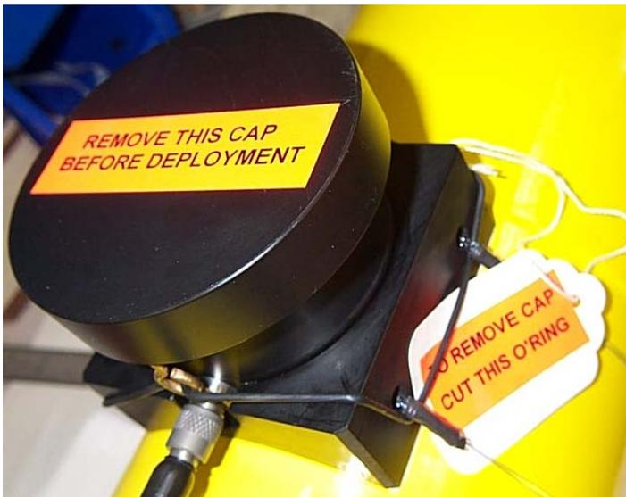
**The Flntu Sensor has a protective cap that must be removed before deployment. To remove cap cut black O-ring which holds it in place.**
