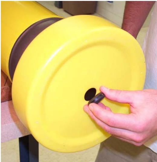
2. Carefully pry black rubber plug out of bottom center of yellow plastic cowling to verify bladder inflation (per below). **Be sure to replace plug before deployment.**
