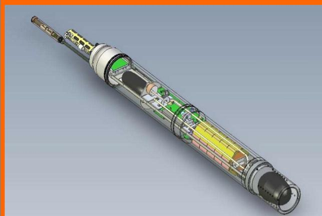
*The PRONUTS prototype is a tool allowing to autonomously profiling the nitrate concentrations in the ocean.
