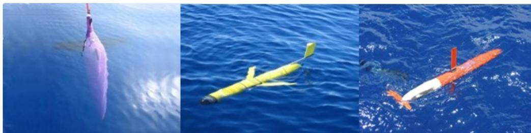
Figure 1: The three operational gliders (from left to right: Seaglider, Slocum, Spray) transferring, while at surface, the data they just collected underwater and receiving new commands thanks to the bidirectional link Iridium link.
